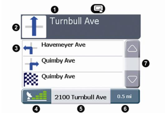
Press the **Navigation** ☰ to cycle to the *Turn-by-Turn* screen. A route must be calculated for this screen to be able to display.
