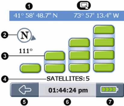
From any navigation screen, tap the GPS icon to display the *GPS Status* screen. This screen provides a visual representation of the GPS information being received.
