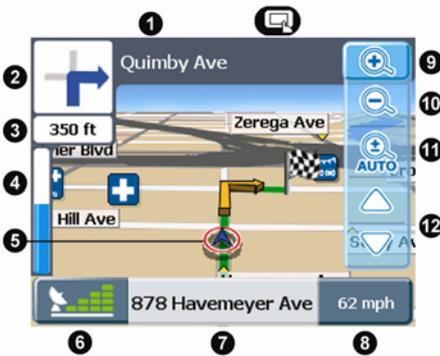
Press the **Navigation** button
