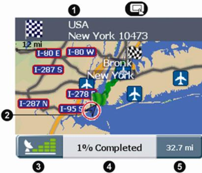
Press the **Navigation** button ☰ to cycle to the *Route Summary* screen. A route must be calculated for this screen to be able to display.
